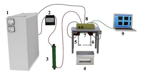
Figure 1. SAD synthesis installation used to produce the carbon nanoparticles soot, power source (1), reference amperimeter (2), ballast resistor (3), cooled stainless steel synthesis chamber (4), cathode (5), anode (6), micro-positioning system (7), automated control unit (8) and PC for data acquisition (9).
