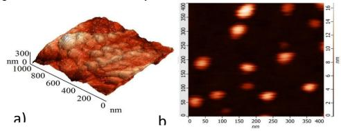
*Figure 3.* AFM studies: a) Height diagram of the non-purified sample, b) Image of the purified sample showing well dispersed CNOs
